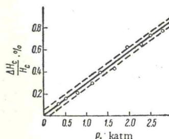
Fig. 3. Relative changes in the critical field values of a  $MnF_2$  specimen plotted against uniaxial pressure applied along the four-fold axis. The broken lines enclose the average scatter values of the experimental points.
